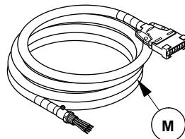
**1 Snap together harness (M) and connect slabs (N & Q)**
